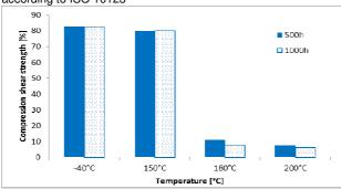
compression/shear strength shaft-hub joint at temperature based on initial value at room temperature measured at determined temperature according to ISO 10123
