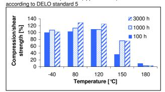
compression/shear strength glass/glass at temperature based on initial value at room temperature measured at determined temperature according to DELO standard 5
