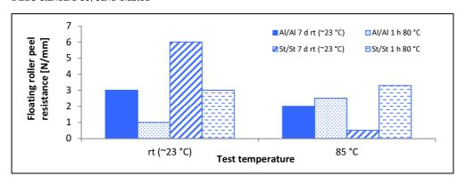
Temperature stability Al/Al DIN EN 1465, sand-blasted component thickness: 1.6 mm
