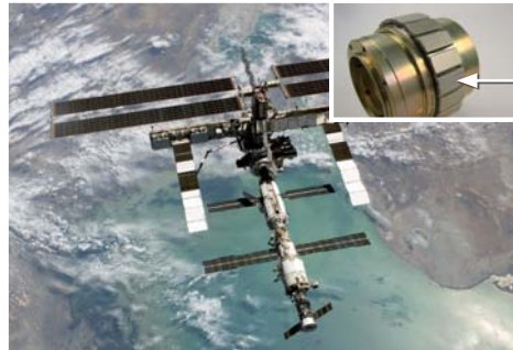
Magnets bonded to a stator of space motors (figure: DLR) for the ISS International Space Station (figure: NASA)
